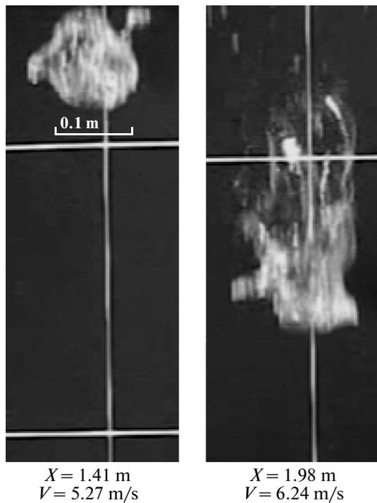
**Fig. 3.** Photographs showing formation of loose expanding body and its disintegration during free fall of a 0.2-l water ball.
