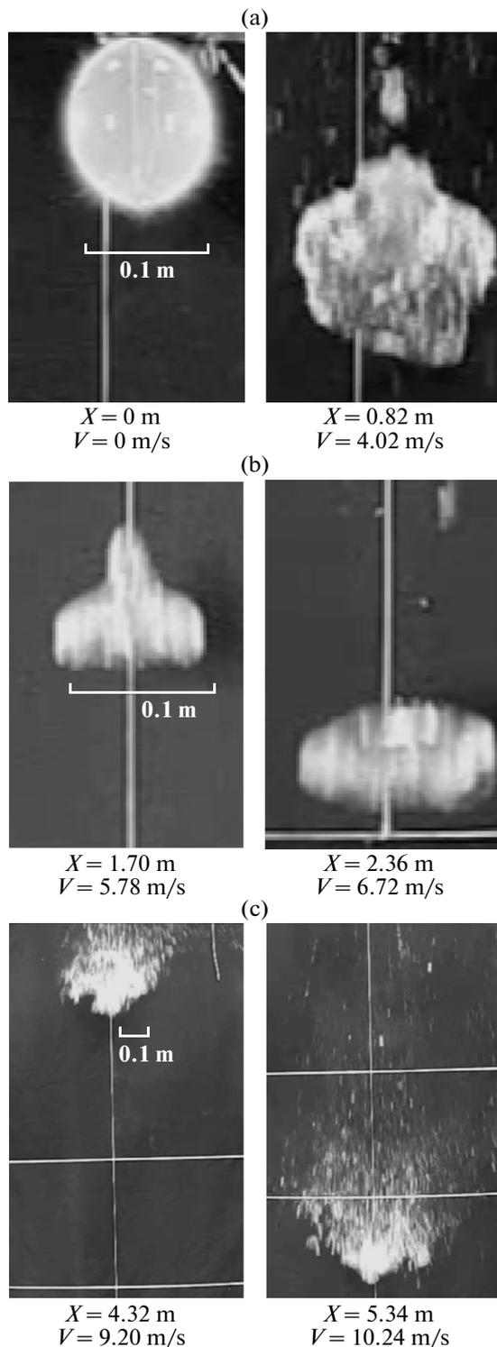
**Fig. 1.** Photographs showing deformation and disintegration of water ball during its free fall in air from an initial altitude of ~5 m: (a) 0.5-l ball,  $X = 0-0.8$  m; (b) 0.1-l ball,  $X = 1.7-2.4$  m; (c) 0.2-l ball,  $X = 4.3-5.3$  m.
