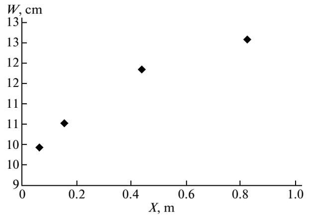
**Fig. 2.** Plot of transverse (lateral) size  $W$  versus traveled distance  $X$  for free-falling water ball with an initial volume of 0.5 l.
